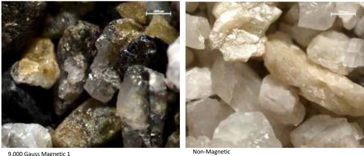
Microphoto images of pre and post extraction of magnetic minerals from the concentrate
