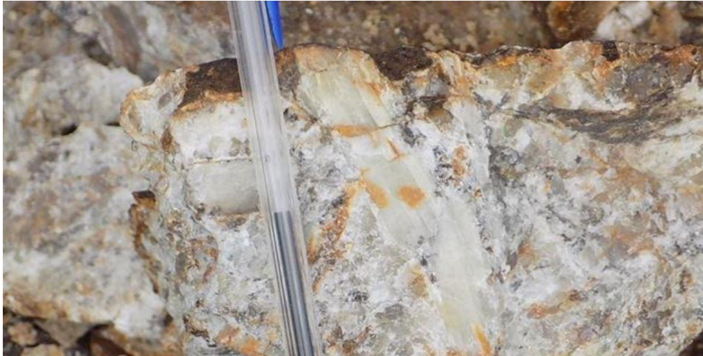
Rock Chip Sample collected showing white spodumene (the large, long prism to right of the blue pen) in a quartz feldspar matrix
