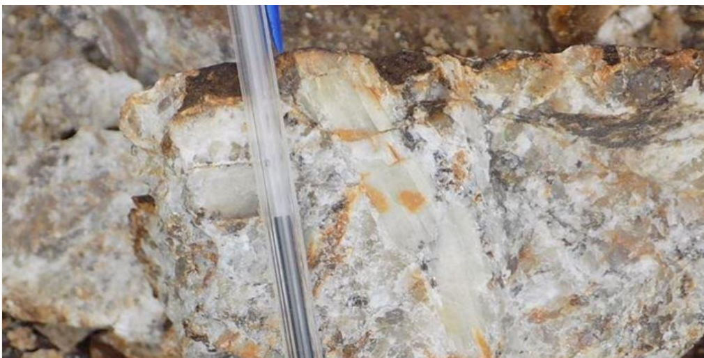
Figure 4: Rock Chip Sample collected showing white spodumene (the large, long prism to right of the blue pen) in a quartz feldspar matrix
