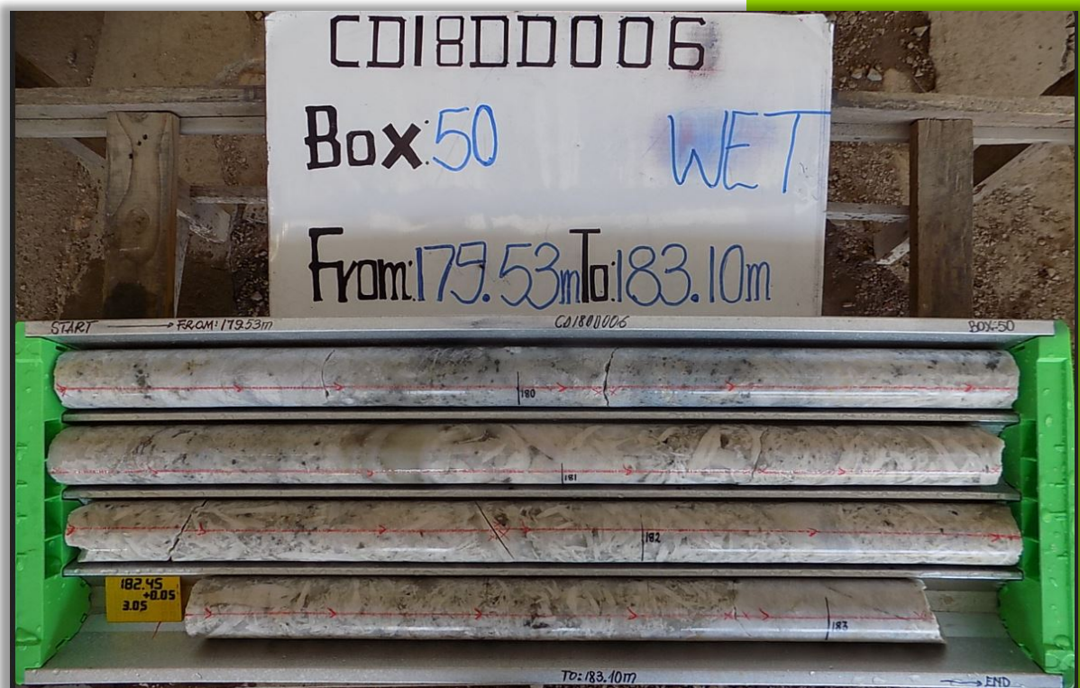
Figure 4: CD18DD006. 181 – 182m 4.65% contained \text{Li}_2\text{O}
