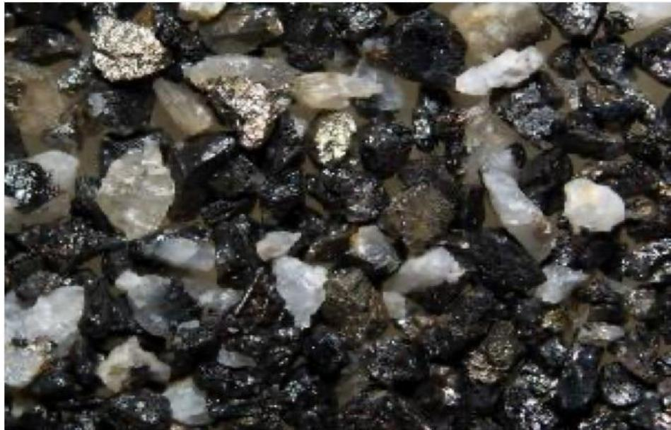
Figure 1: Coarse tin concentrate 0.5 to 8mm
