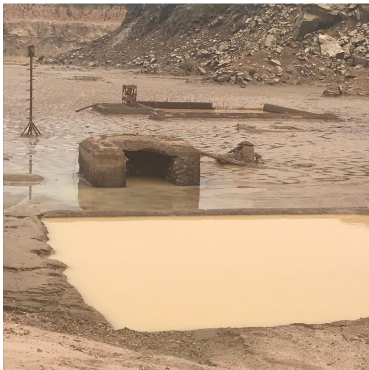
Figure 11: The sump on the floor of the Roche Dure pit, post dewatering
