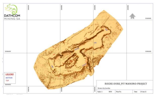
Figure 2: Processed digital terrain model for the Roche Dure pit
