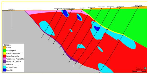
Figure 5: Cross section showing the weathered pegmatite relative to the fresh pegmatite
