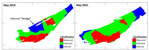
Figure 4: Plan view at 590 m elevation, showing the comparison of the Mineral Resource classification
