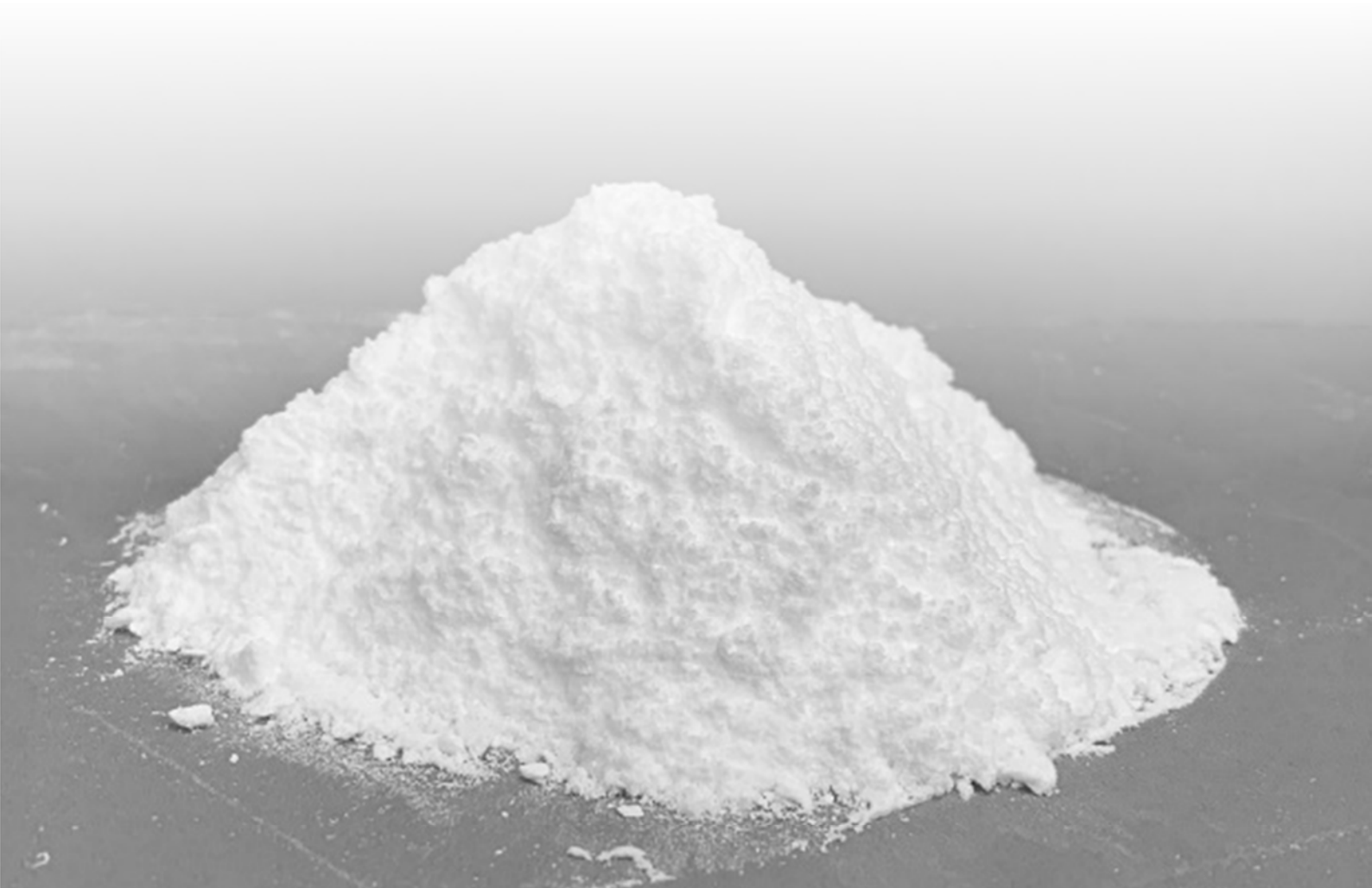
Primary Lithium Sulphate produced from Roche Dure SC6 under metallurgical testing for AVZ's planned Manono Lithium Sulphate Plant
