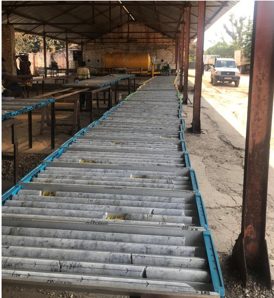
Figure 2: Top 3 rd of drillhole MO22DD001 down to 124.6m laid out for lithological logging
