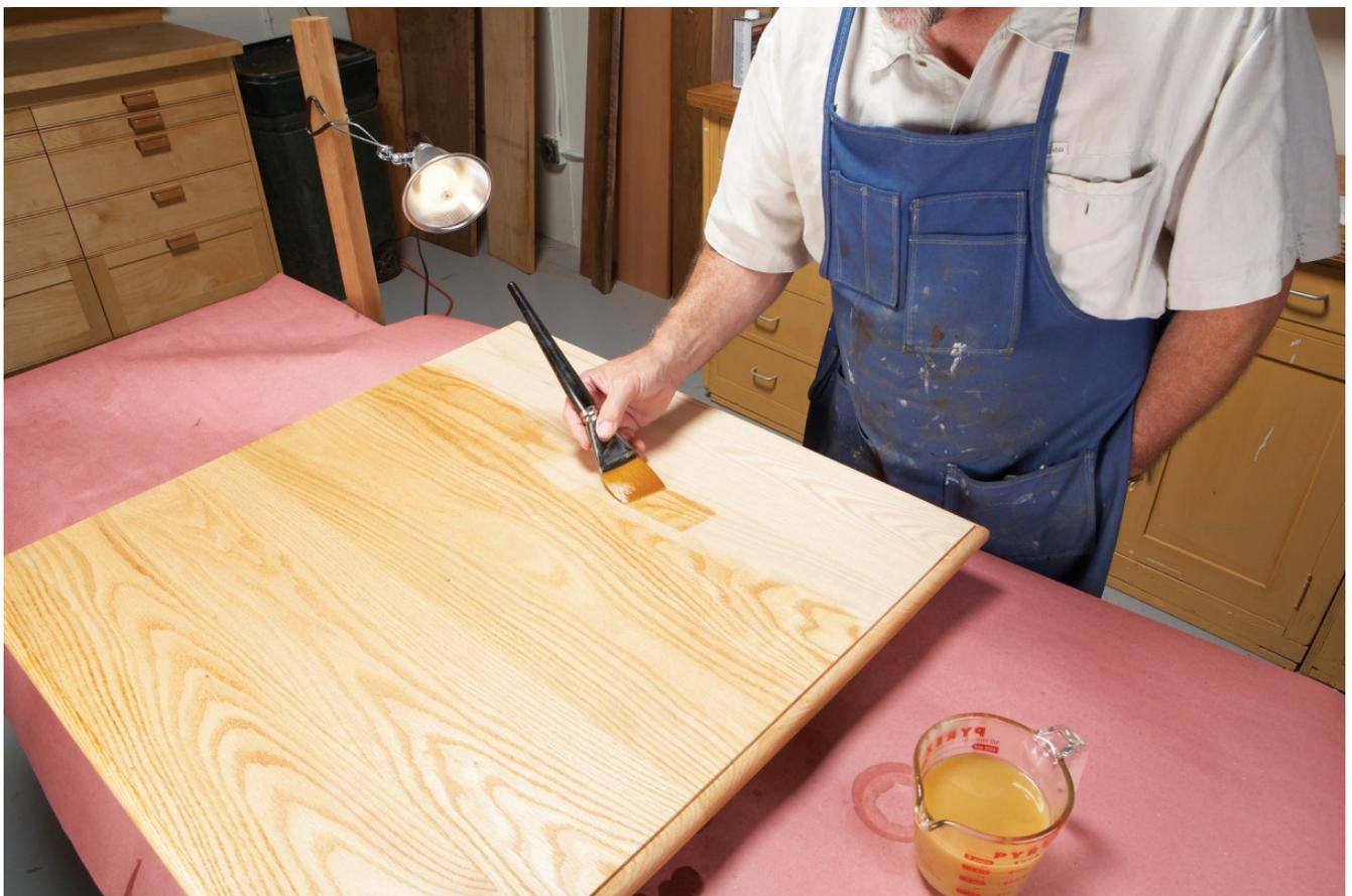
*Overlap your strokes on a large surface. Any time you re-wet the brush, land the brush in a dry area. Use a back and forth stroke to blend the new stroke into the wet shellac ahead of it and beside it and lift off right at the edge to avoid snapping the bristles over the edge. Lifting off prevents pools of shellac from being left at the edge and turning into drips.*
