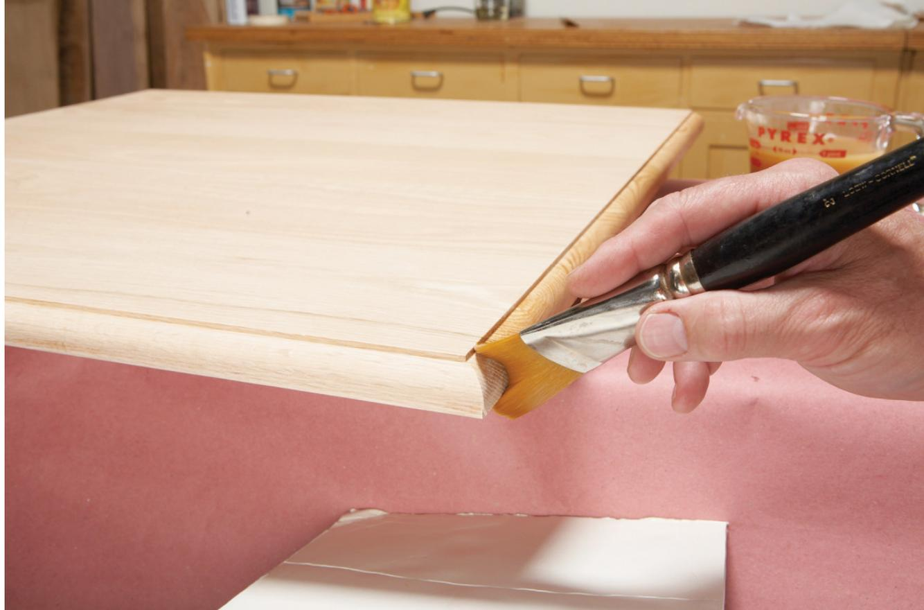
*Come back to finish the bare spot where you started the stroke. Think of your brush as an airplane. Land the brush near the unfinished end and then lift off right at the edge to avoid snapping the bristles over the edge. Lifting off prevents pools of shellac from being left at the edge and turning into drips.*
