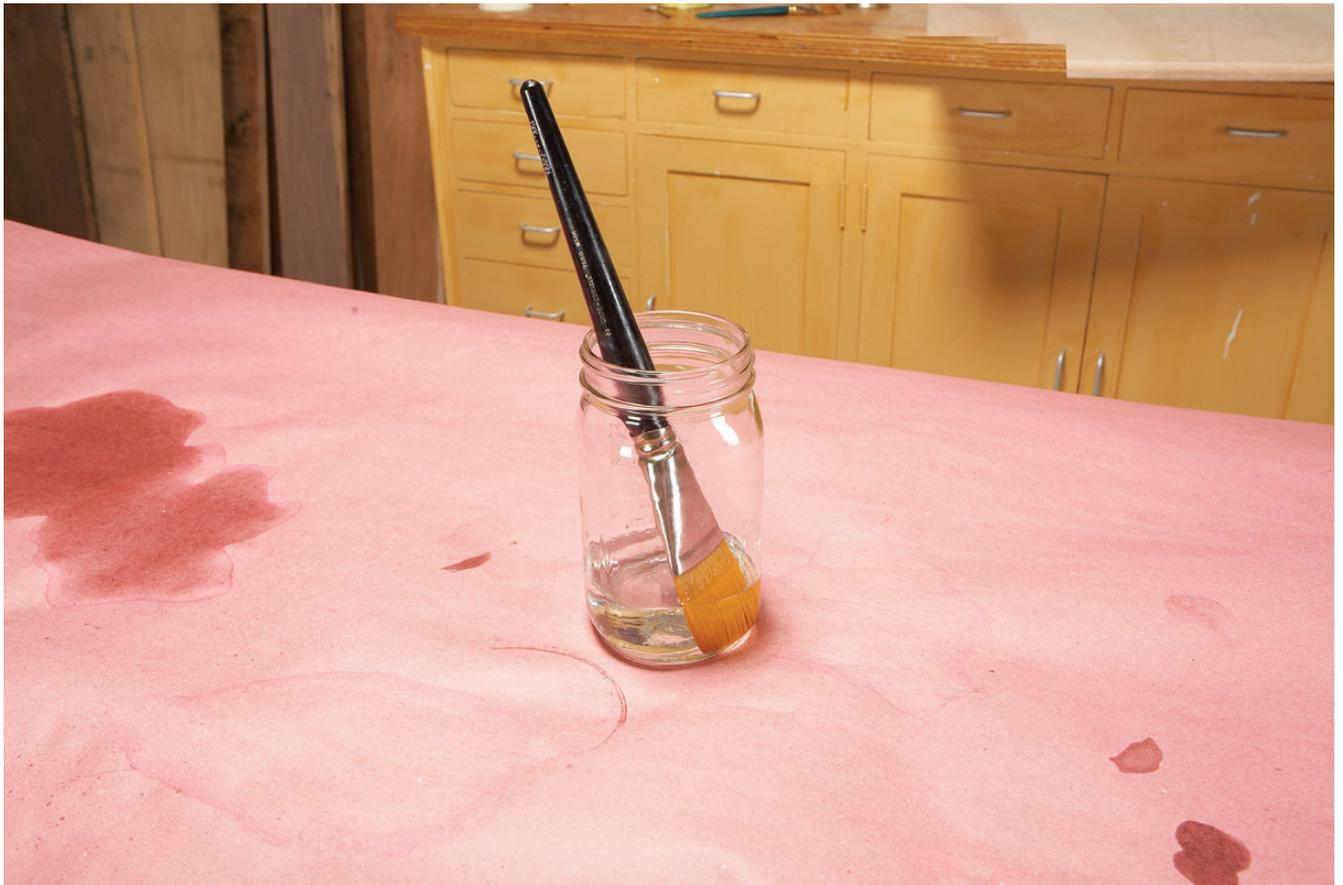
*Charge the brush by soaking it in denatured alcohol for a few minutes before use. This helps the shellac flow better from the brush.*
