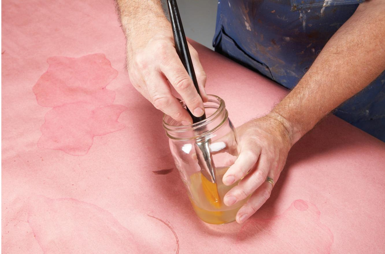
*When the brushing is over, cleaning your brush is a breeze. Just swish it around in a container with clean denatured alcohol. This will clean out most of the shellac from the brush. Unlike varnish or water-based finishes, it's okay to leave some residue in the brush.*
