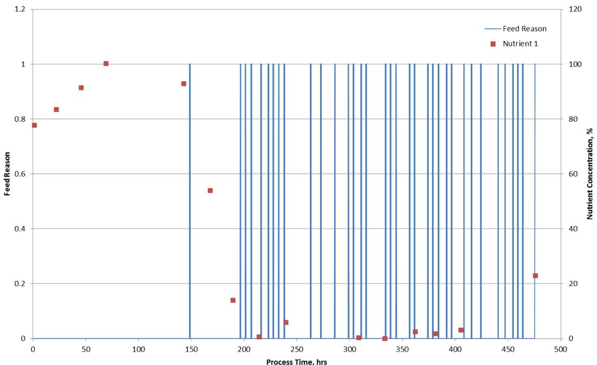
Figure 6. Feed Reason (pump on/off) and Nutrient 1 concentration.
