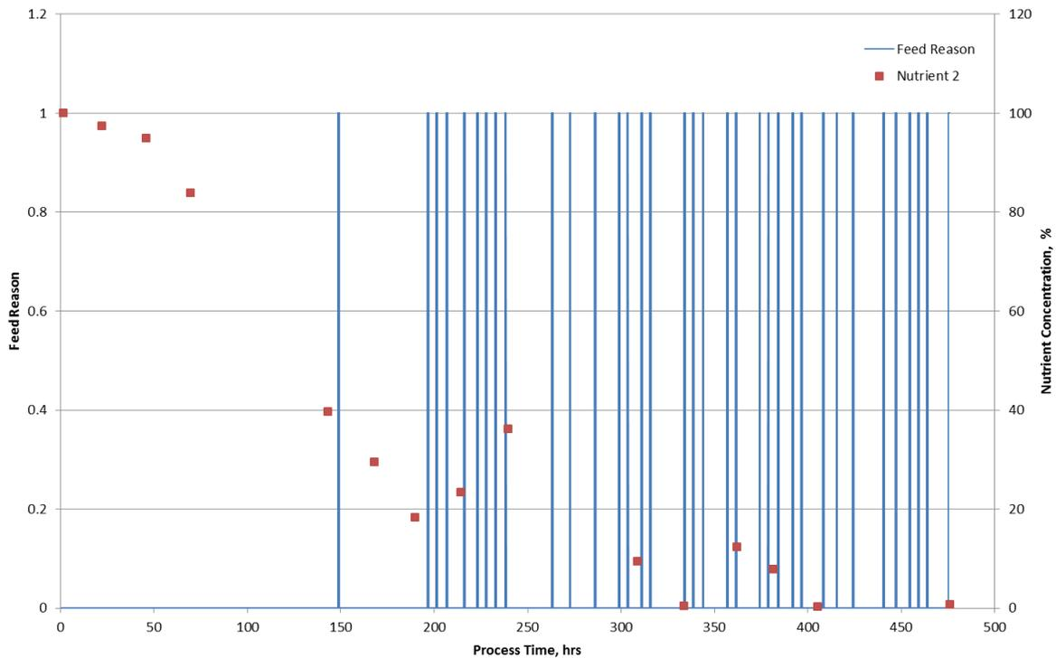
Figure 7. Feed Reason (pump on/off) and Nutrient 2 concentration.
