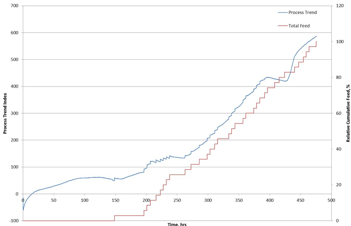
Figure 2. Process Trend Index and cumulative feed profiles generated during AFC of a CHO cell culture.
