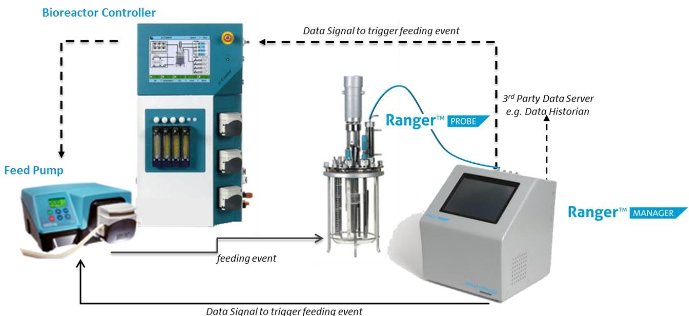
Figure 1. Typical Ranger system setup for AFC of a benchtop bioreactor, showing Probe, Manager and direct connection to feed pump.
