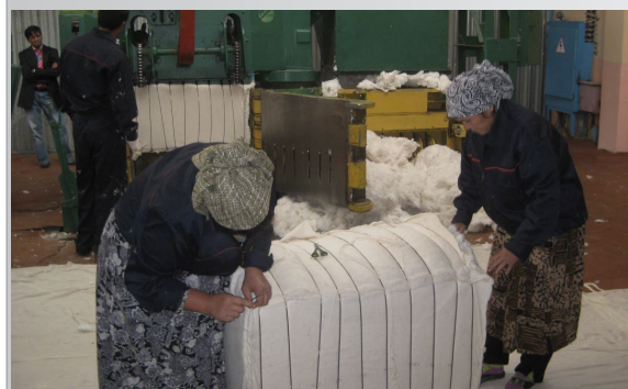
Figure 5.2: Pressed cotton fiber being hand sewn into a bale at a gin in Uzbekistan. (V. Gurney)
