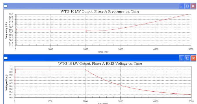
Fig. 7. Island with 10-kW Output, 16-kW Load, Under-voltage Trip in 0.96 s.
