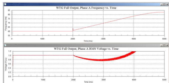
Fig. 6. Island with 65-kW Output, 10-kW Load, Over-frequency Trip in 0.2 s.
