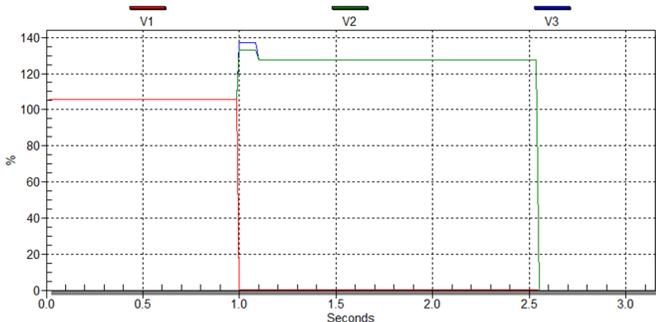
Fig. 5. Temporary Overvoltage (TOV) Limited with Unbalance Detection.
