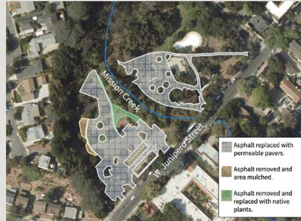
Aerial view of the now completed Oak Park Storm Water Infiltration Project (City of Santa Barbara)
