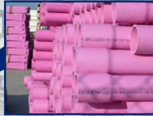
Recycled Water Pipeline
