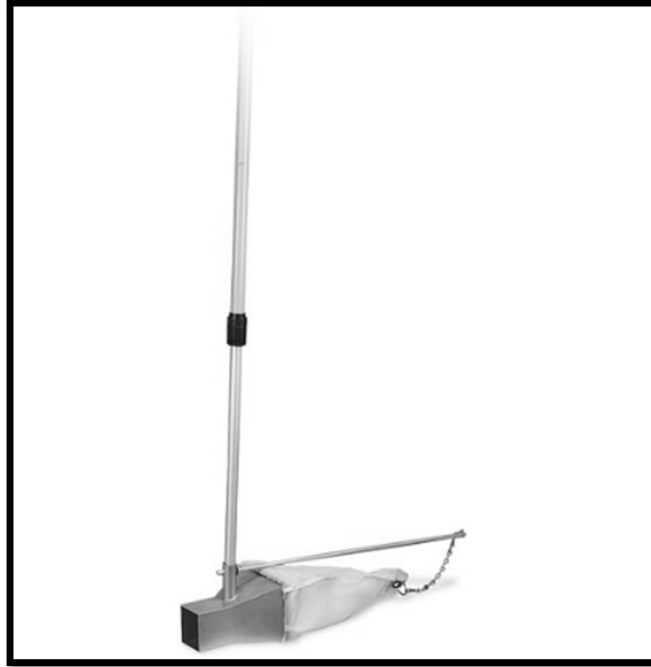
Figure 18. Helley- Smith bedload sampler.
