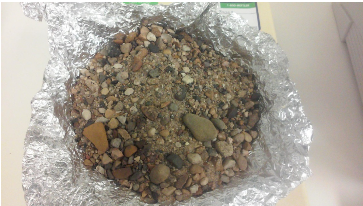
Figure 26. Bedload of Station 4 of Indian Mill Creek (September 8, 2016).
