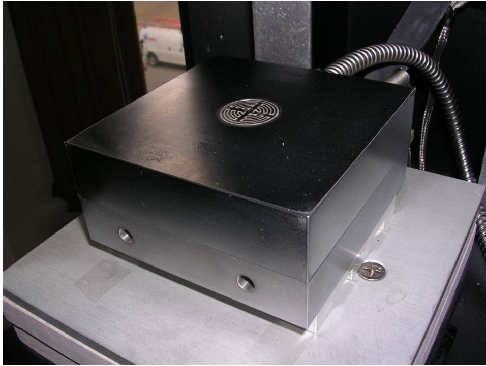
Figure 10-1 Ceramiccomb-1” reusable sensor embedded in press platen
