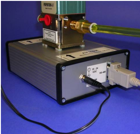
Figure 2 LTP-303 Rear Panel Connections
