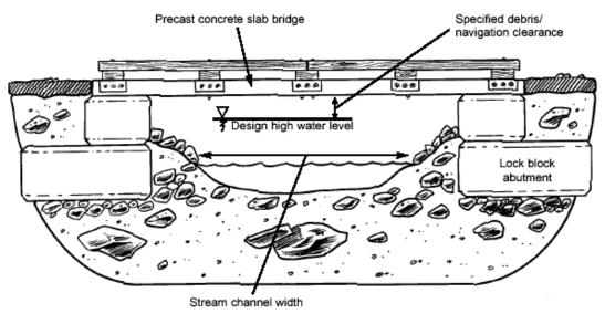
**Figure 1b. Example of a clear-span bridge.** A clear-span bridge is a structure that spans the stream's open water channel and does not involve the construction or installation of any structure between the stream's banks.
