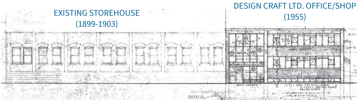
1955 Building Permit drawings by Bregman & Hamman showing the east elevation of the Design Craft Limited Office/Shop at 342 Dufferin Street and the existing storehouse building to the south at 340 Dufferin Street (City of Toronto Building Records; Annotated by ERA).
