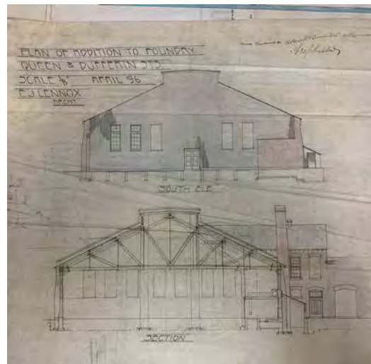
April 1896 south elevation and section of 358 Dufferin Street, the “foundry” building, as drawn by E.J. Lennox. Today, this south elevation is either partially obscured by the core oven building, or since demolished. The pitched roof has since been replaced with a flat roof (E.J. Lennox Fonds, Archives of Ontario).*
