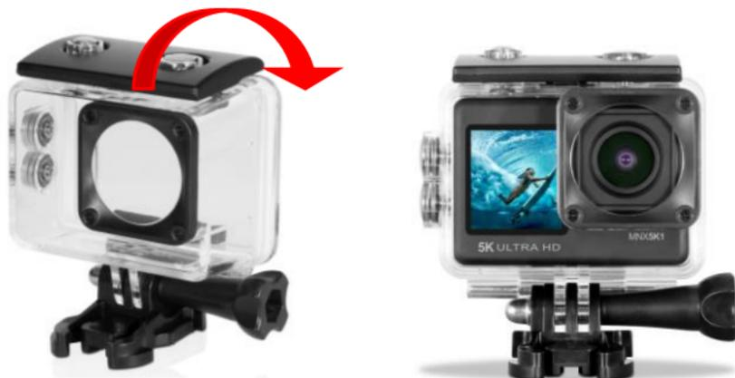
Once the camcorder has been placed into the waterproof case, close the rear door, then latch the edge of the lock onto the rear door and then push down on the front edge of the lock it into place. **Please note: To avoid injury, make sure your fingers are not in any of the openings or under the lock.**
