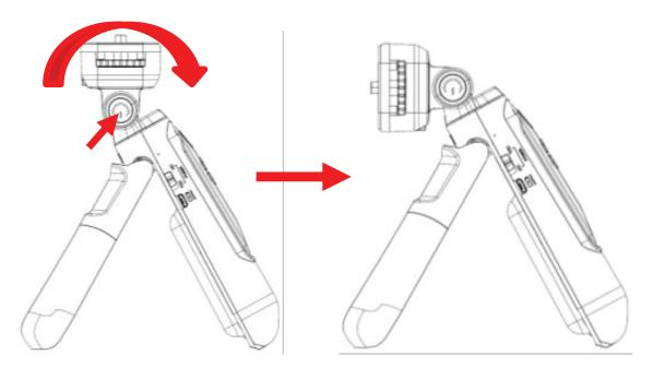
The camera mount can also be rotated horizontally, simply push in the
