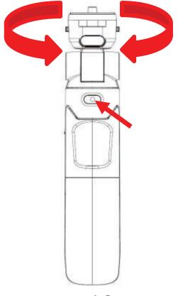
horizontal rotate mount button and then rotate the mount to the position you desire. The camera mount can be rotated a full 360°.
