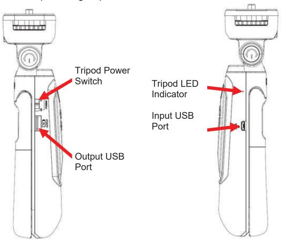
To charge the tripod, simply plug in the small end of the USB cable into the USB port on the tripod labeled "Input" and the larger end of the USB cable into the AC adaptor. When charging, the LED indicator on the tripod will flash red, when it is fully charged, the LED indicator will light up solid red.
