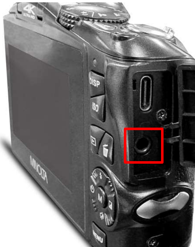
3.5mm Microphone Input Port
