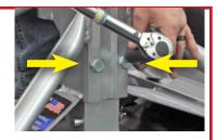
**2-1**. Place the Ultimate Connection base in the bed of your truck with the Ultimate Ball closest to the tailgate. You can use your bed grooves to square up the hitch before tightening it down.
