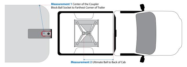
1-2. If Measurement 1 is SHORTER than Measurement 2 then you might be close to having perfect clearance. However, "perfect clearance" is not really necessary for 5th wheel trailer towing, most truck/ trailer combinations work great with 60°-70° turning clearance. If you want more details about turning clearance, watch the short video clip on our website at the link below (or scan the QR code).
