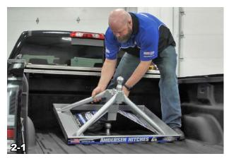
**♦ IMPORTANT** Ensure that the coupler tube set bolts are loose enough to allow free movement of the coupler tube.
