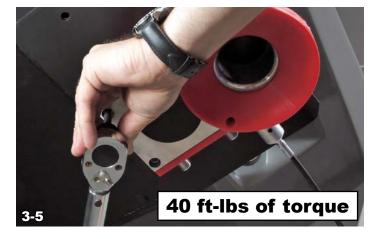
**NOTE:** Because kingpins vary in height, some blocks will have space between the coupler block and the kingpin plate (as shown at right) while others will be flush. This is normal and does not affect performance at all.
