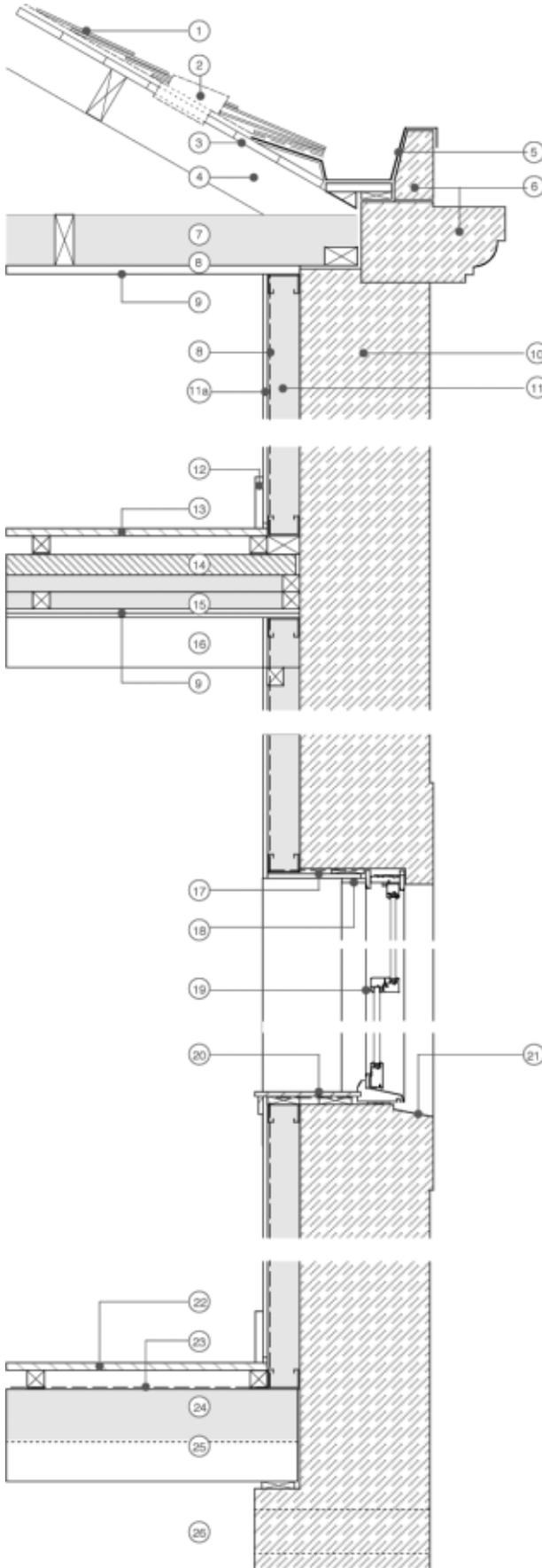
1. Existing slates taken up and replaced, nailed through breather membrane with stainless steel nails.
