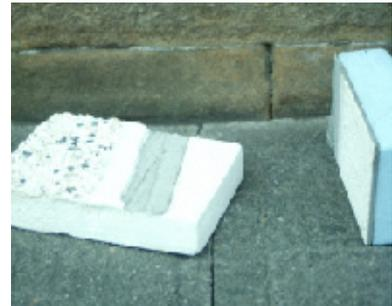
Bonded external insulation systems are difficult to recycle or re-use.
