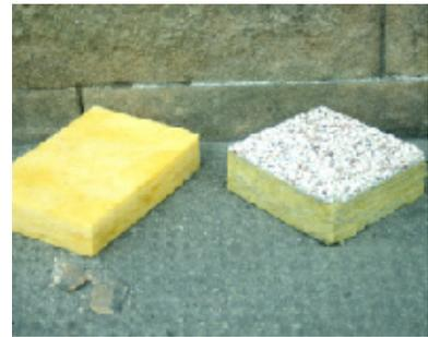
Flexible insulation bat on the left offer greater potential for re-use.
