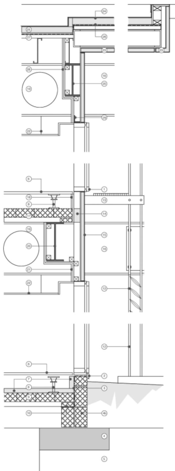
27. Profiled metal deck with Z purlins (j) mechanically fixed @ 600mm centres
