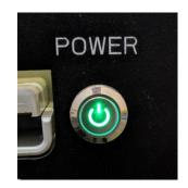
In order to use the ePower battery this button must be in the on position to either charge the battery or operate the vehicle. If this button is in the off position neither charging nor driving will be possible.
