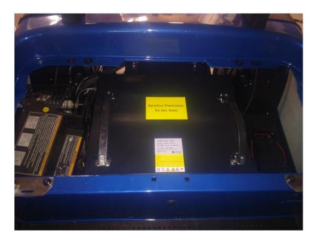
Once the ePower batteryis set in the battery tray the lifting straps can be removed.
