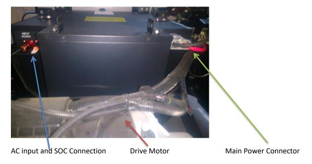
F) Optionally, the included state of charge indicator can be installed on the vehicle where desired. The state of charge gauge has four LED's which represent 25% increments of the batteries available charge.
