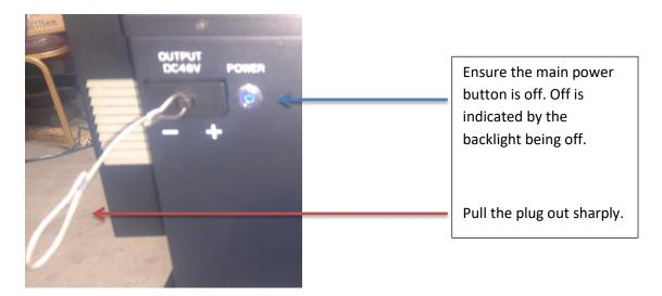
The ePower comes with a pre-made main power harness. For this step ensure that the main Power button is in the off position, the back light will not be lit. Connect the ring terminals of the main power harness to the vehicles existing positive and negative connections. Plug the connector in to the ePower DC 48V output by firmly pressing it in to the ePower until the connector click in to place.
