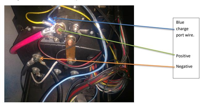
A blue wire goes in to the vehicles existing charge port. This wire will need to be moved over to the main vehicle positive. The main contactor is a convenient location to connect this to.
