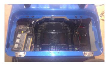
Lead acid batteries removed and tray is clean and dried.
