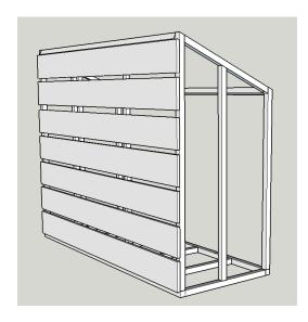
Attach the boards on the side. When you get to the top boards. You can cut the angle after attaching the board with a circular saw. Or you can clamp the board in place, make a pencil line then cut the board on your work table.
