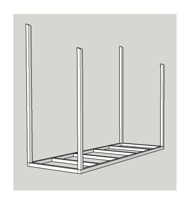
Line up two of the 30" pieces and mark for the correct length. Cut them at a 22.5 degree angle on both sides and attach with glue and screws.
