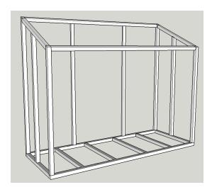
Measure for the roof supports. These should be around 30" and they don't have any angles since you twisted the stretchers in step 4. Glue and screw them into place. The frame is now complete! Don't worry if it doesn't feel sturdy, screwing on the outer boards with take care of that.
