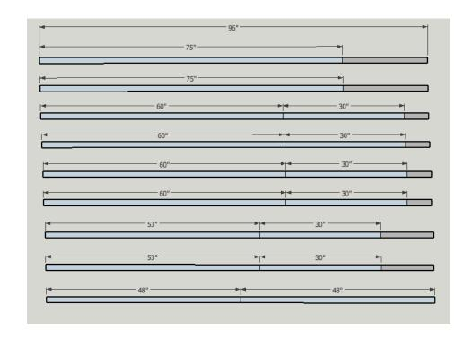
All the 60", 53" and 48" pieces have a 22.5 degree angle cut on one side of them. 2 of the 30" pieces have a 22.5 degree angle cut on both sides of them. (It's best to cut these pieces to fit when it is time to assemble them to get a perfect fit.)
