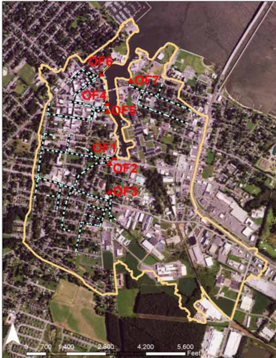
Cambridge Creek Stormwater Model
