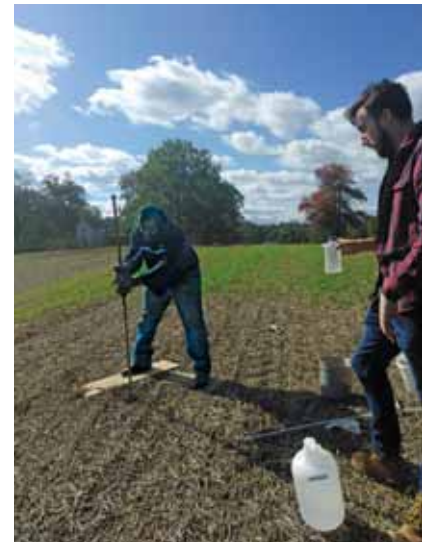
University of Maryland students install a lysimeter to monitor nitrogen levels in groundwater. Photo credit: University of Maryland
