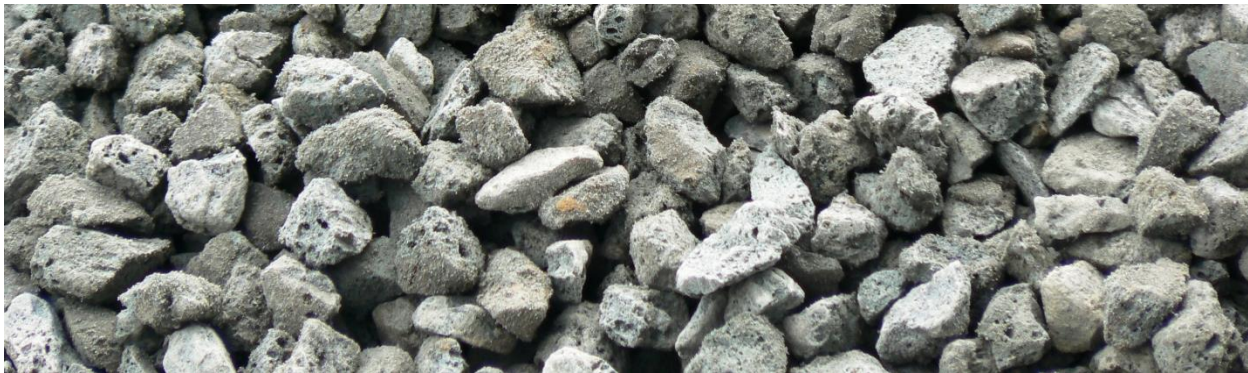
Figure 2 Stalite Lightweight Expanded Slate Coarse Aggregate
