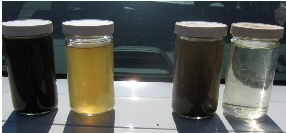
Figure 13 (From left) Charlotte Mecklenburg Bioretention Soil Mix Influent & Effluent; Stalite Bioretention Media Influent and Effluent (2010)
