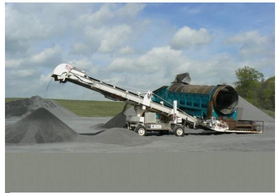
Figure 6 The Trommel and Belt Screening System at Stalite Plant - Gold Hill, NC
