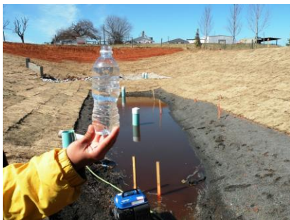
Figure 15 First Flush Capture from Cistern at Hospice of Wake County - Raleigh, NC (2010)
