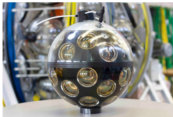
Figure 16. The KM3NeT optical module. [93] The optical module consists of a glass sphere with a diameter of 42 cm, housing 31 photosensors. The glass sphere can withstand the pressure of the water and is transparent to the faint light that must be detected to see neutrinos.
