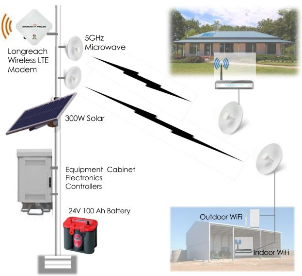
The **LongReach Wireless HighPoint** solution when coupled with the LongReach Wireless (LRW) ODU provides Internet connectivity to dwellings, out buildings and remote properties where 4G wireless connectivity is currently unavailable or signal quality is too weak to support reliable and effective Internet. Experience has shown that many rural and regional properties may have a "high point" location where good quality 4G wireless signals can be received and sent.
