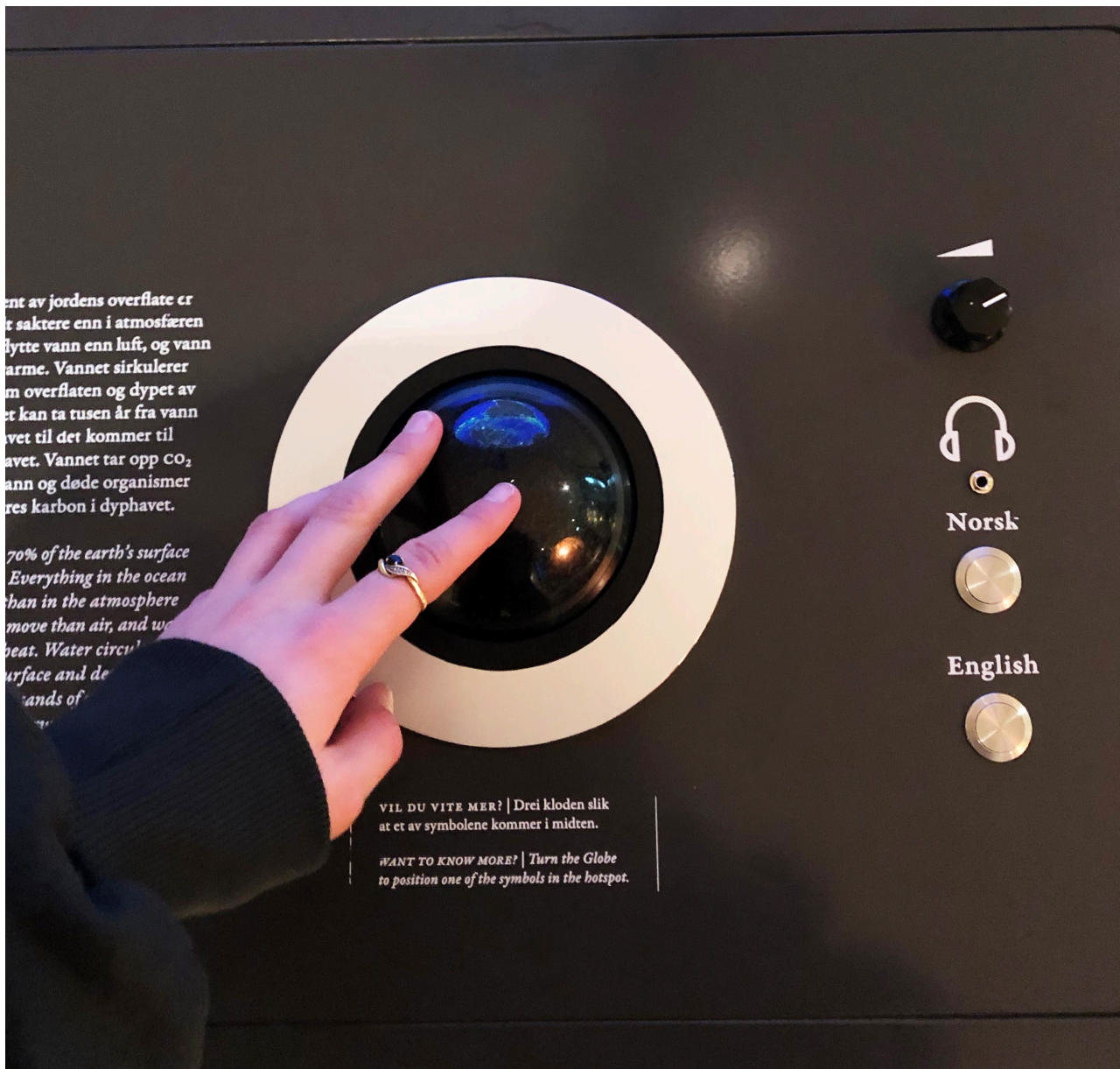
Figure 4: One of the control panels showing the navigation ball, volume switch, headphones input and buttons that allow you to switch between Norwegian and English language.
