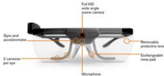
Figure 6: Illustration showing the eye-tracking glasses specifications (Tobii Pro, 2020a).
