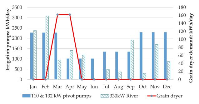
FIGURE 5: MONTHLY AVERAGE ENERGY DEMAND FOR EACH SITE: RIVER PUMP (SITE A), PIVOT PUMP HOUSE (SITE B), AND GRAIN DRYER (SITE C).
