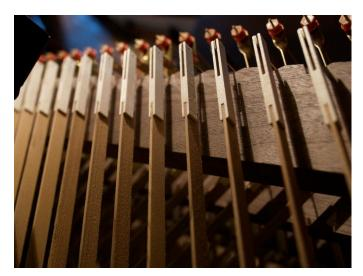
This ancient system gives the organist intimate control over the speech and release characteristics of the pipes for a sensitive control of musical phrasing and articulation. Careful design and construction promises longevity measured in centuries. In this organ, the action is a suspended key action, in which the keys are hinged at the rear and literally hang from the valves (pallets) in the
