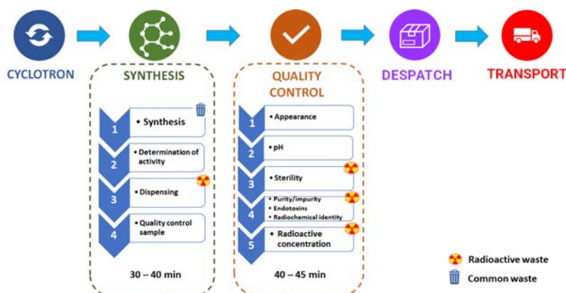
Figure 1. Diagram of the synthesis process and quality control of ^{18}\text{F} FDG
