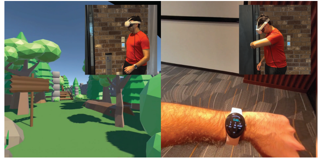
Figure 2: A user exercising in a virtual nature trail (left) can view their fitness tracking data when looking at their smartwatch via dynamic passthrough (right).
