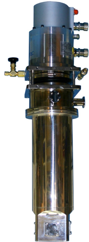
The above picture shows a cryocooler with a vacuum shroud, radiation shield, and sample holder installed.
