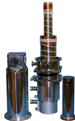
The above picture shows the DE210 Cryocooler installed on the GMX-20 interface with the vacuum shroud and radiation shield removed.
