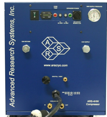
The above picture shows the compressor for the system. What is not shown is a required vacuum pump, Helium Hoses (included with system), temperature controller and Helium Gas bottle with regulator for the exchange gas.
