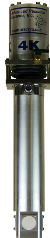
The above picture shows a cryocooler with a vacuum shroud, radiation shield, and sample holder installed.
