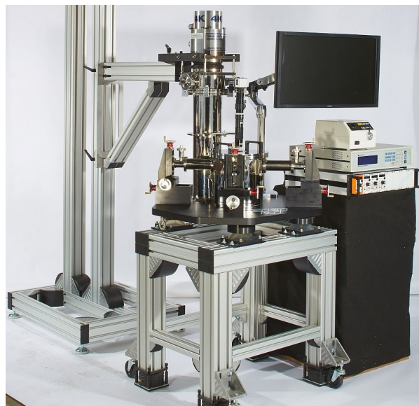
Fig 2. The above picture shows the probe station with optional floor table, piezo controller, as well as standard temperature controllers, monitor, cryocooler stand, and light source. Ideal configuration should employ pneumatic optical table for best vibrations.
