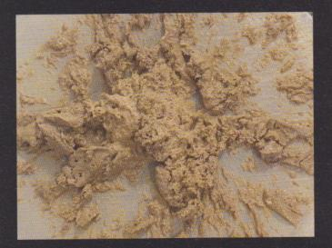
push the resin towards the middle of the bag in as small a puddle as possible to facilitate collecting.
