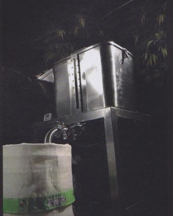
There is often a lot of leaf matter in the bag which happens most frequently with small leaf material (sugar trim) and is due to the need to maximize the exhaust flow; merely put the collected leaf matter back into the machine and clean the bag thoroughly with alcohol if there is any stickiness. The cleanliness of the meshes defines the amount of trichomes that can pass through the sieve into the Collection Bags.
