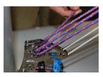
Continue to feed the Dyneema control line back up to the double block, feeding the line from front to back.
