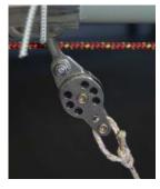
2 Tie the length of **Vectran V12** (1.45 m) in a bowline loop through the top block.
