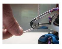
Thread the V12, previously attached to the top block, through the pulley/becket from the top.
