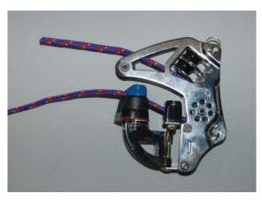
Take the length of Dyneema race control line (4.5 m) and thread it through the Harken base unit before you attach it to the mast as shown. Ensure that the tail is underneath the horizontal pair of blocks.
