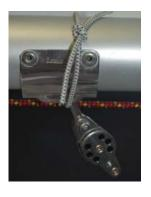
Put the top block and tang onto the boom and tie the small length of shockcord in a loop as shown to stop the top block from coming off the boom unintentionally.
