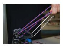
Feed it through the double block from the bottom of the block and through the non-becket side. Make sure the becket is on the port side.
