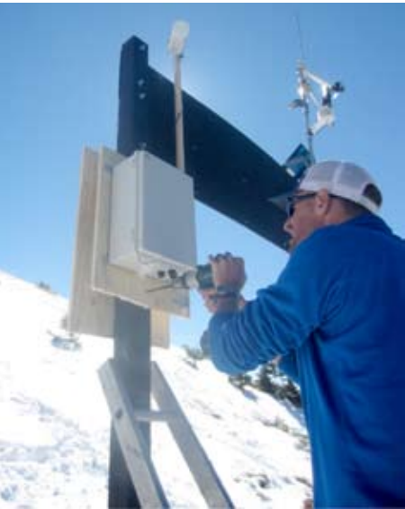
A-Basin veteran ski patroller Devon Haire installs a wireless AvyNode on a trail sign.
