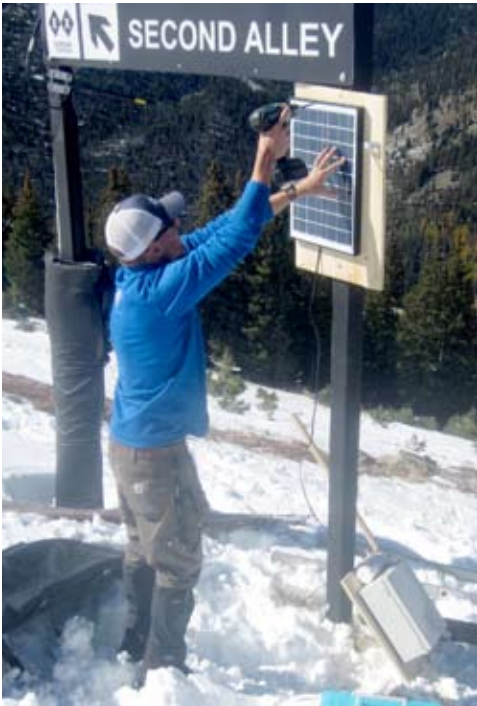
A-Basin veteran ski patroller Devon Haire installs a wireless AvyNode on a trail sign.
