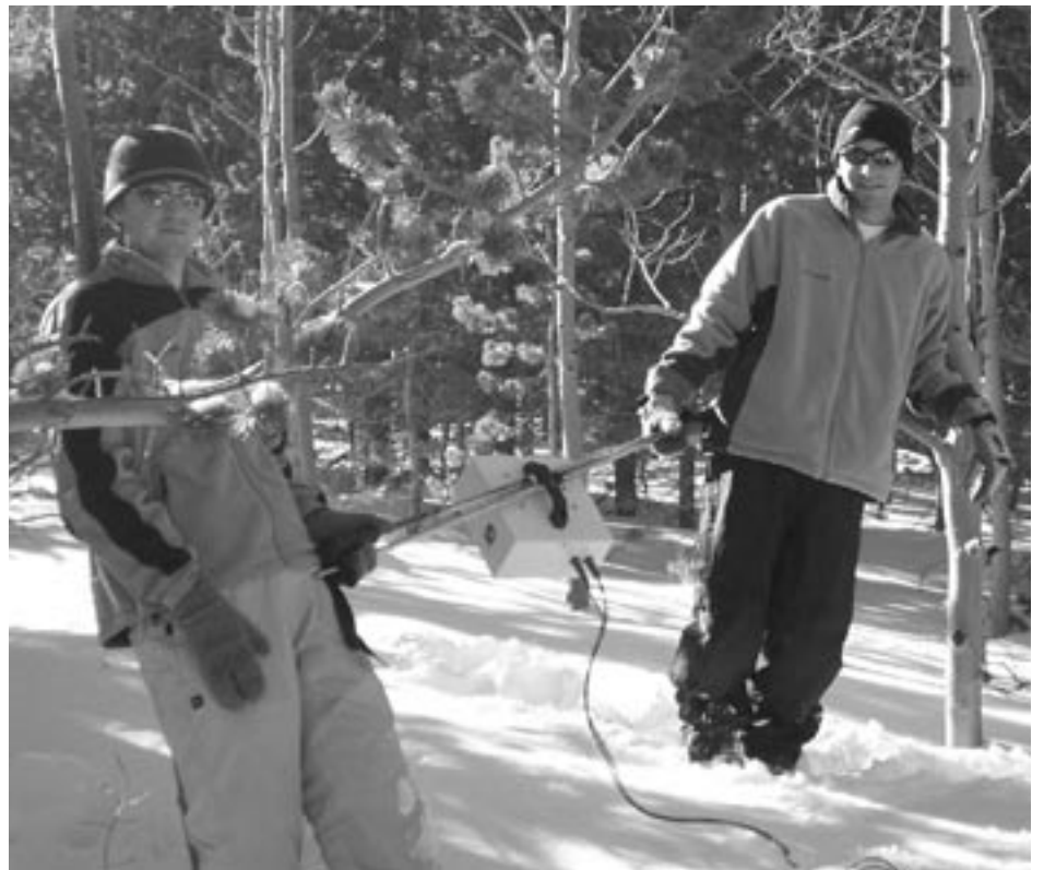
High school students Paul Kirschner and Austin Williamson make measurements with the new light-weight portable radar. The small battery and laptop used to acquire data are not shown.
