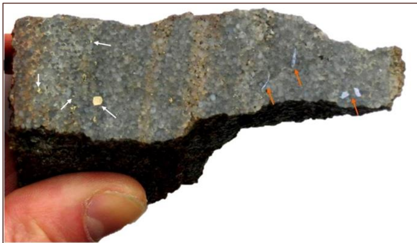
Source: Haugaard (2011) (2). Note: The white arrows denote chalcopyrite, and the red arrows show bornite with chalcocite rims. This sample had a grade of 0.74% Cu and 16 g/t Ag, although similar material returned grades of 2.35% Cu and 59 g/t Ag (2).
