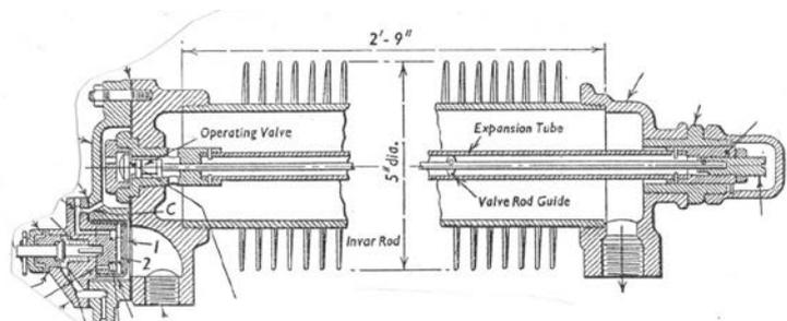
*Diagram 8. Carriage heating element*
