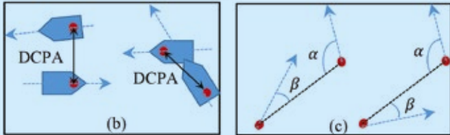
Fig. 2. CPA-based determination of situational awareness, main parameters and limitations. A CQS and a physical accident may develop early before TCPA as shown in (a). (b) shows DCPA safety limits have different interpretations depending on the type of encounter between vessels. Pose at CPA in (c) does not ensure accurate situation assessment with symmetrical safety evaluation functions. CPA ignores vessel manoeuvrability in an encounter, and COLREGs-defined responsibility.
